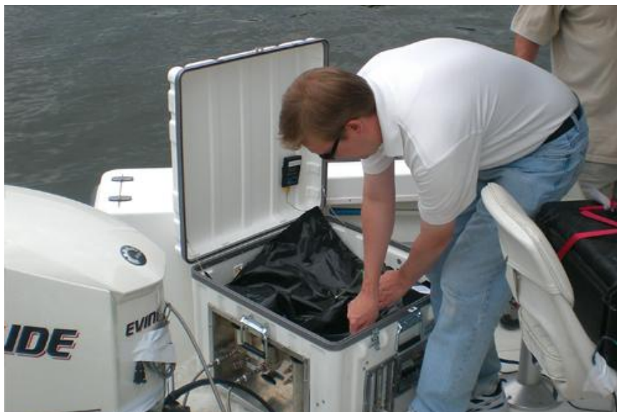
Evinrude engineer Jeff Wasil loads a fresh emissions-trapping pouch into the Marine Portable Sampling System (MPSS) that he designed.
